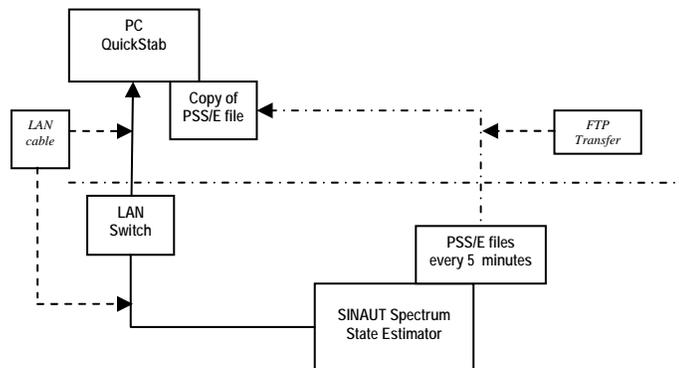
**Figure 1:** Schematic description of the interim implementation of real-time stability assessment at NOS BiH
