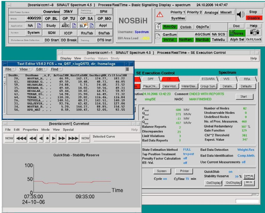
Figure 6: Visualization of real-time stability analysis results in the SCADA/EMS user interface
