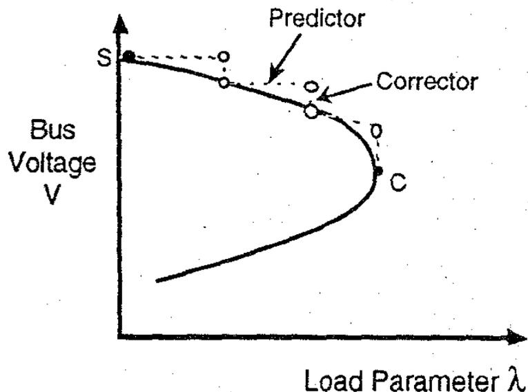
Figure 8: Steps of the Continuation Power Flow method
