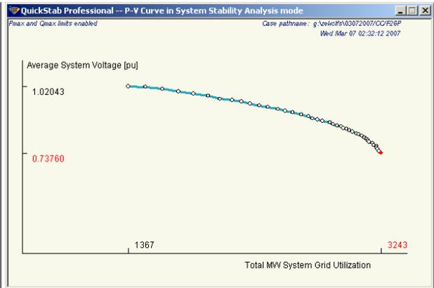
**Figure 3:** P-V curve depicting the case worsening process -- the average system voltage decays while the total MW system grid utilization increases up to the point of voltage collapse
