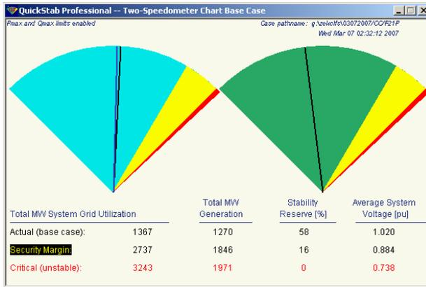
**Figure 2:** Two-Speedometer Chart depicting the distance to instability (red) and to the security margin (yellow)
