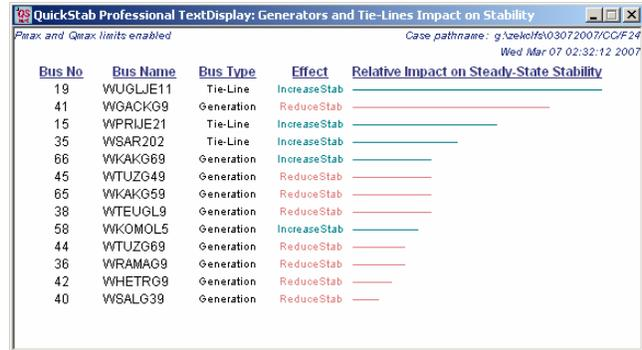
**Figure 4:** Unit ranking bar chart depicting the impact of generators and tie-line injections on stability
